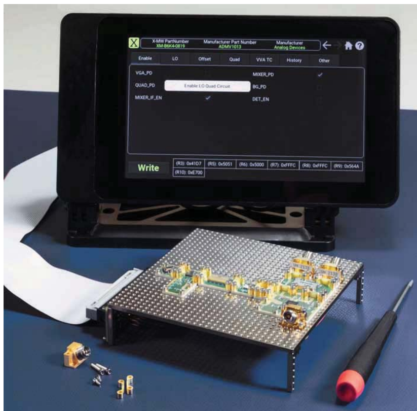
4. The XM-RDK-201/ADMV1013 frequency-upconversion kit from X-Microwave provides components needed for upconversion of RF signals in the range of 24 to 44 GHz.
